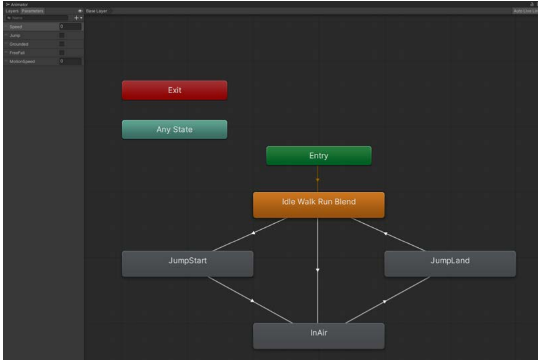
An example of an Animator state graph: Compare its structure with a StateMachine.
